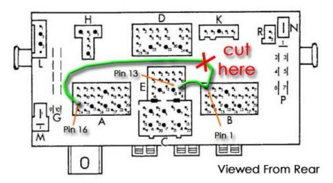
6. There's a couple of blue or green wires that run to terminal B1. One of the wires runs out to A16, the other to E13. Cut the one that runs to A16. Cut it at a point about 1" from where it exits terminal B1.
