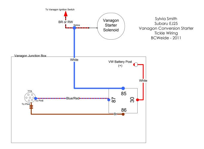
Starter Tickler Wire had .3 volts at engine idle (after starting). Installed relay to limit feed to 12 volts only during startup. Eliminates cycling idle in drive/reverse at standstill.
